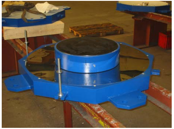
Fig. 17: Sizes of spherical steel isolators, any other intermediate sizes are possible
