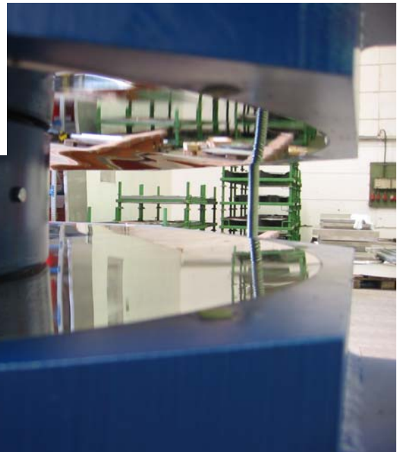
Fig. 18: Assembly of a SIP-D Type devices with perfect concave stainless steel sliding surfaces
